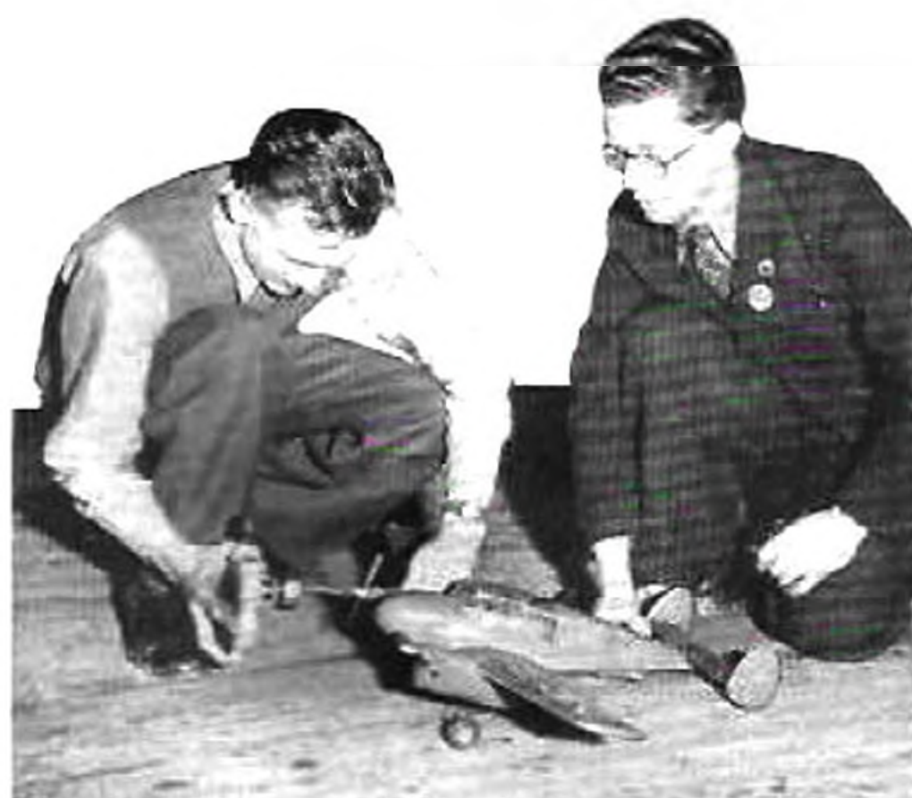
Len Gabriels, assisted by W. Archer, prepares to start up his C/L "Gemini" in the arena. He designed and constructed two .4 c.c. diesels for this model. Note the ultra high-g geared winder type starter.
