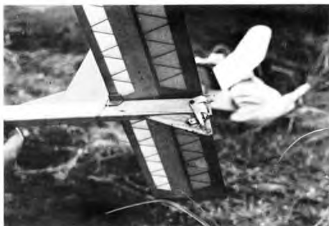
About a half second after the rudder is activated, the stab is allowed a small amount of negative incidence for glide set-up.
