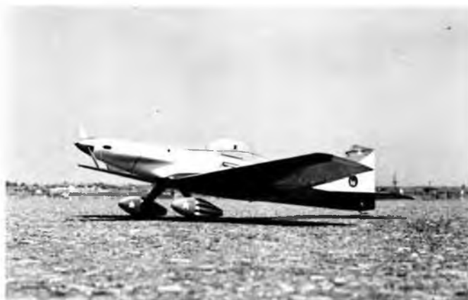
Paul White's ST .15 powered K & K Ballerina QM pylon racer. Ship weighs 3 lbs., has 306 sq. in. wing area, and flies in mid 90's.
