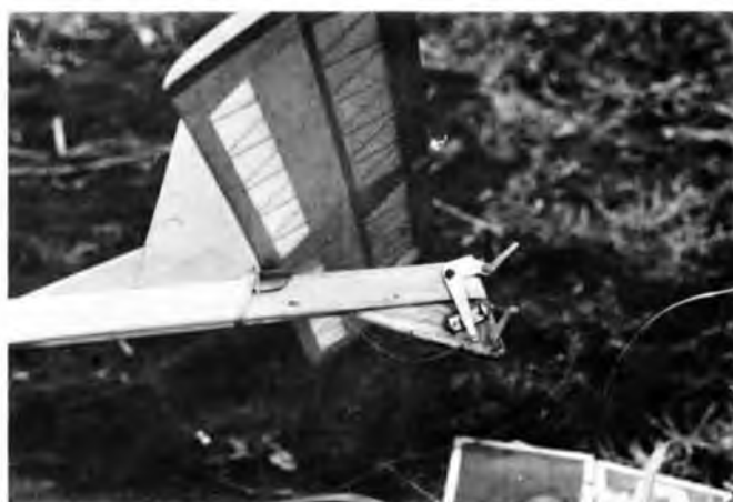
The last step occurs three minutes after the plane is released, when the stabilizer pops up to 45 degrees for dethermalizing.
