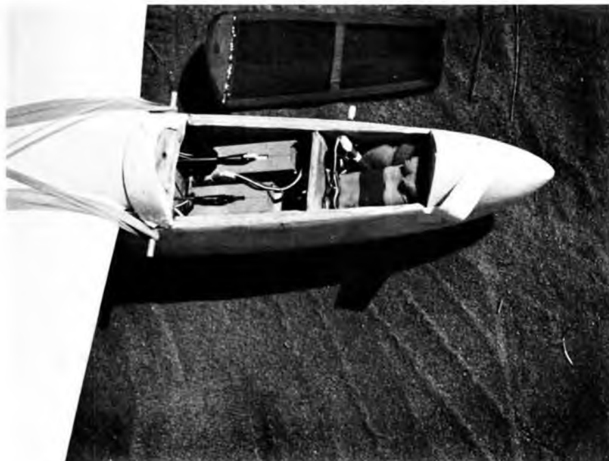
As indicated on the plans, here is the installation of the "Ancient Bonner Servos" in the luggage compartment. The "Band-Aid" holds the front end of the canopy in place, a dowel at the aft end.
