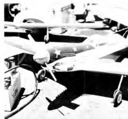
Jack Stafford's P-51 FAI ship with Goldberg retracts and Murphy muffler on K & B engine.
