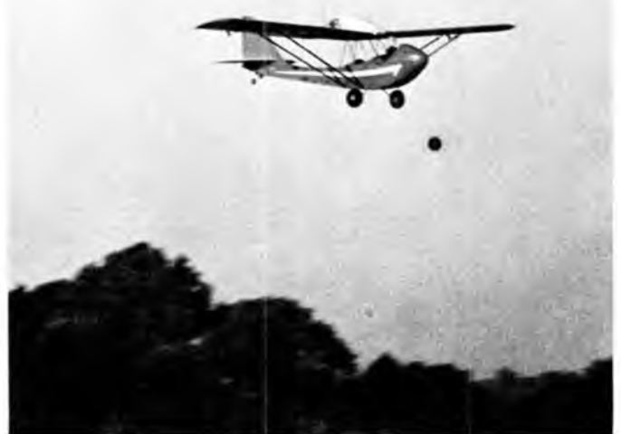
Another scale job from Delaware, this one the Curtiss Wright Pusher, span 75", O.S. 30! Three are flying in club. Lands at 12 mph.
