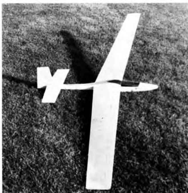
Our columnist Le Gray's "Scorcerer", with turbulators on wing. Tests with sheeted L.E. wing were poor until turbs were added.
