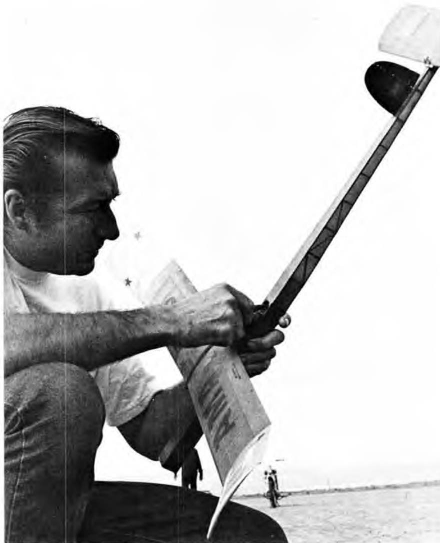
Here's our Free-Flight M.C. extracting a broken motor from his Coupe D'Hiver. Plans on next page...a good airplane to use for breaking in to rubber F/F competition. Note undercamber.
