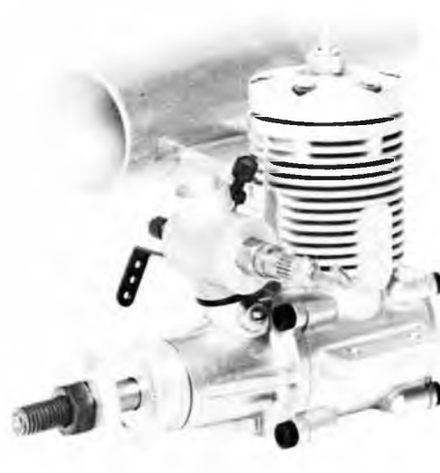
The HP40FR develops .90 horsepower and comes with muffler. Could be used in place of a .60 in some airplanes.
