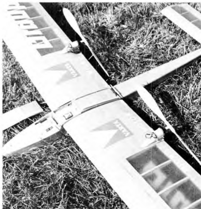
A close-up of the battery-powered R/C job flying above. Varta Deac cells supply 7.2 to 9.6 volts for the electric motors. R/C shut-off for soaring.
