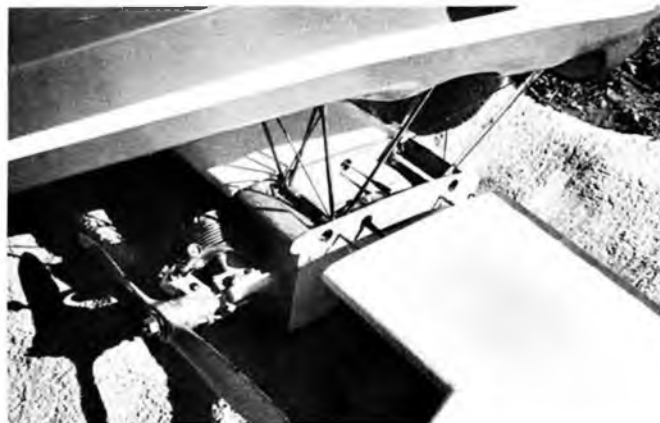
Right wing is now attached, aileron clevis hooked to crank. Wing held on by rubber bands to cup hooks. Power is Enya .35.
