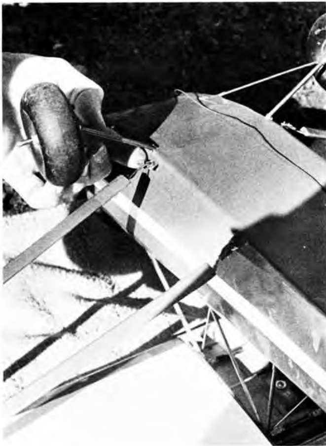
Functional wing struts are hooked on using Rand keepers. "Z" bend in 1/16 inch wire provides adjustment for length. Note receiver antenna.
