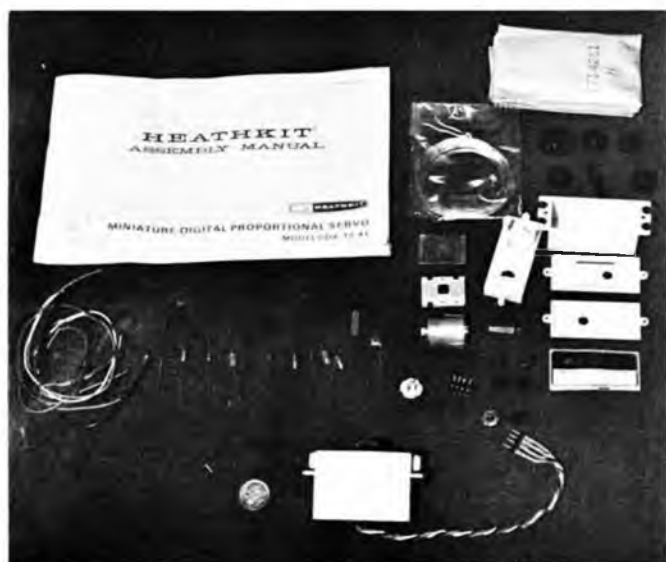
Contents of Heath GDA 19-41 servo kit spread out for examination. Note how few electronic parts go into the amplifier.
