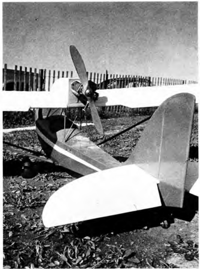
Here's a good view of left-hand prop. You can get left-hand cranks for some engines, but carving a prop isn't bad. It'll last for ever.
