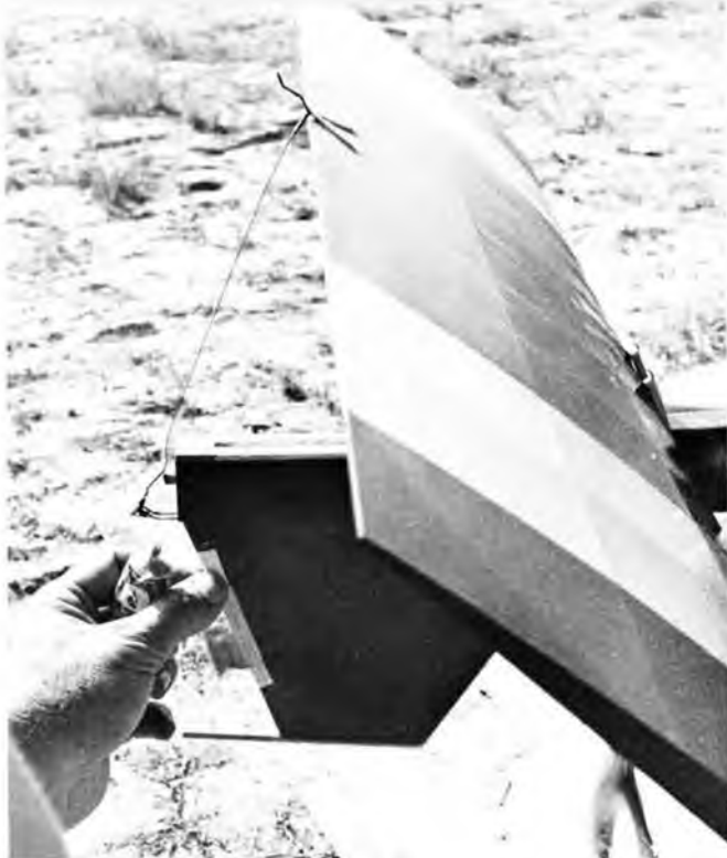
Bob Isaacson is adding a trim tab to his 900 Star Duster. Note stranded wire stop for DT position on stab. Taibi's design is popular kit.
