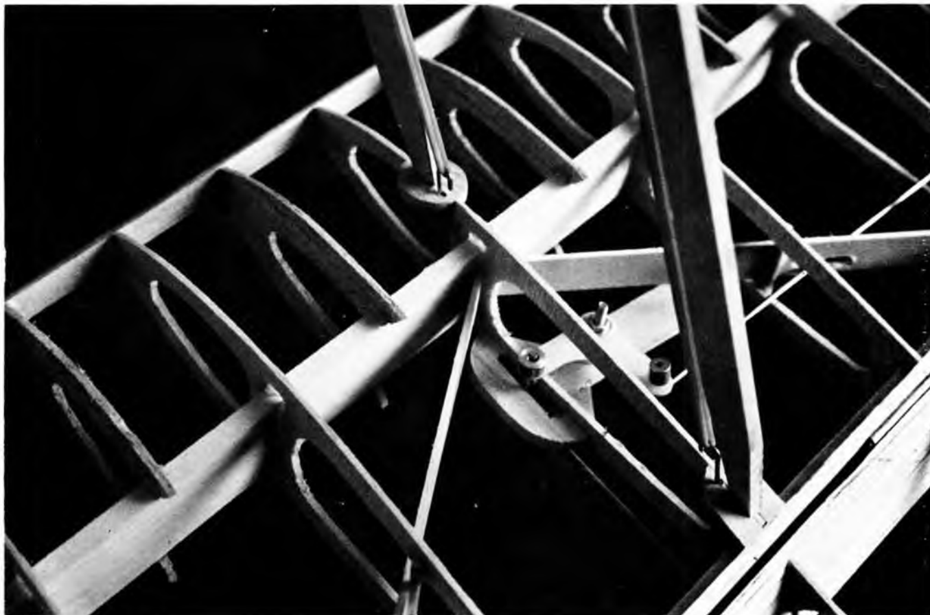
Framework shot of our "Spruce Goose", designed to see if we could build a light airplane out of mostly spruce construction. This one came out at 6-3/4 pounds ready for takeoff! Balsa version was published in M.A.N. Redrawn plans for S.G. will be available soon. Hartman makes FG cowl.
