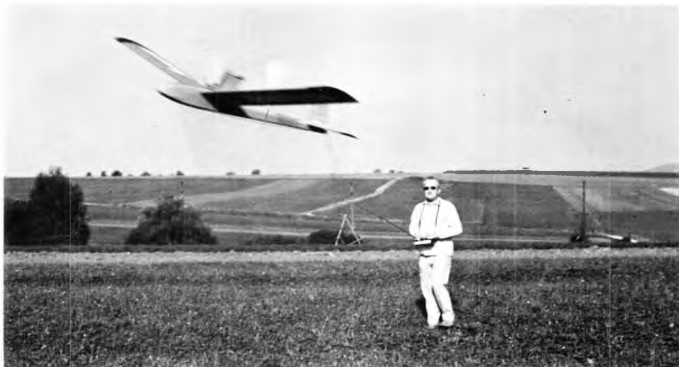
Fred Militky flying the electric powered R/C model that he demonstrated at the World Championships. Plane spans 63 inches and is powered by two Micro-Mo motors turning folding rubber powered type props. Weight is about 2 pounds. Radio is Grundig Varioprop by Graupner.
