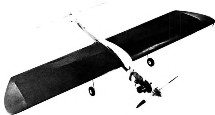
This quickly built stunter was described in last month's "Workbench" column but there wasn't room for the photo. It's John Garabedian's "Trophy Trainer" with foam wing. Uses 40 engine.
