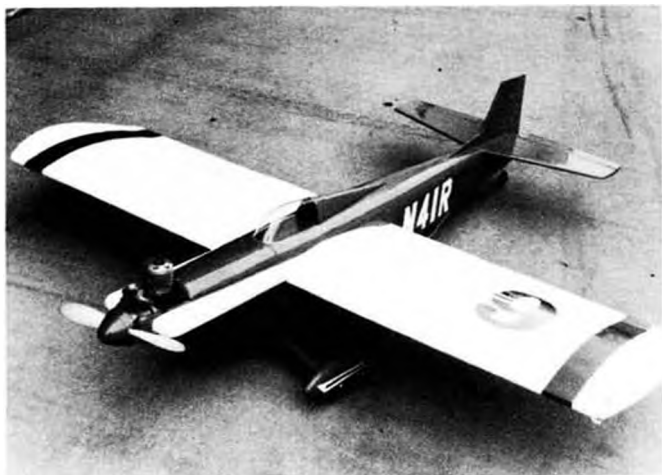
Fred's "Miss Cosmic Wind" is Supertigre powered. He finds the best prop for this engine is a 7x4. Uses K & B 500 fuel.
