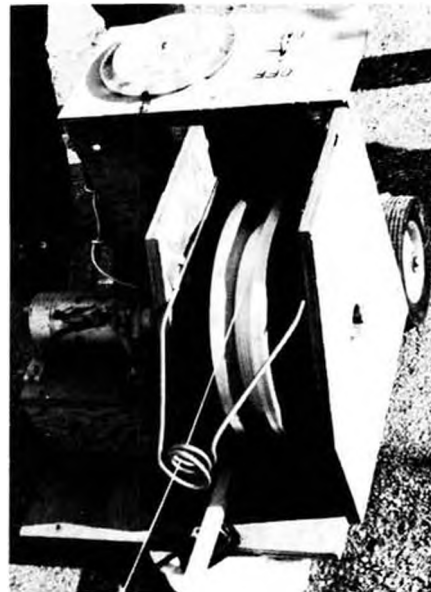
Typical auto starter and battery powered electric winch with "Dial-a-voltage" selector.
