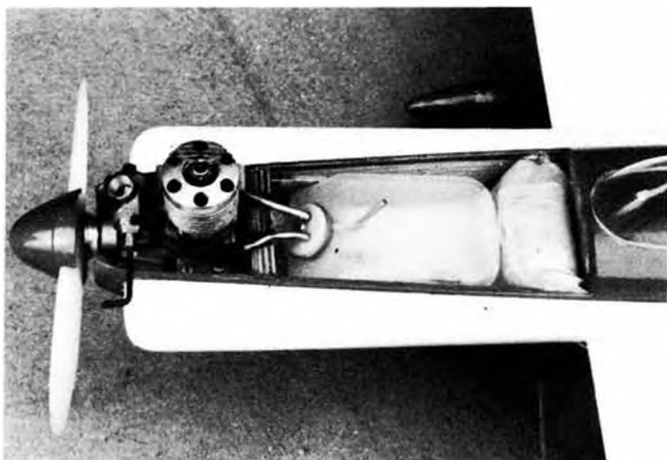
This picture just about tells all as far as the engine and tank installation are concerned. Note carefully wrapped and padded battery pack.
