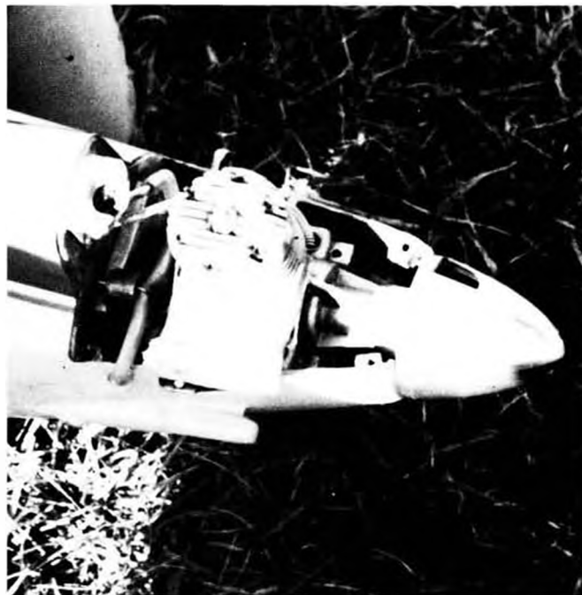
Close-up of Jack Fehling's fuel pinch-off on left rudder command. It saves weight and 40 bucks! Seen at Tangerine races. Good idea.
