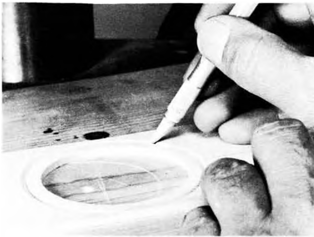
The center disc was cut completely through with the Pawood tool. Now a sharp model knife removes the "square" tire from the stock.
