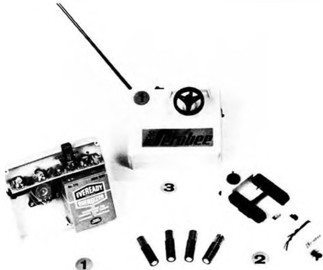
The complete Jerobee radio unit. It's a two-channel proportional set and is under 100 milliwatt....no license required. Range is over 200 ft.
