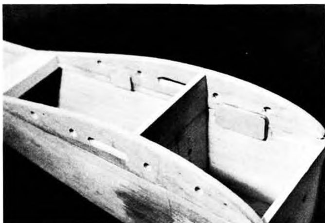
Close-up of uncovered center section, showing rugged construction. Wire wing rods actually suspend fuselage between plug-in panels.
