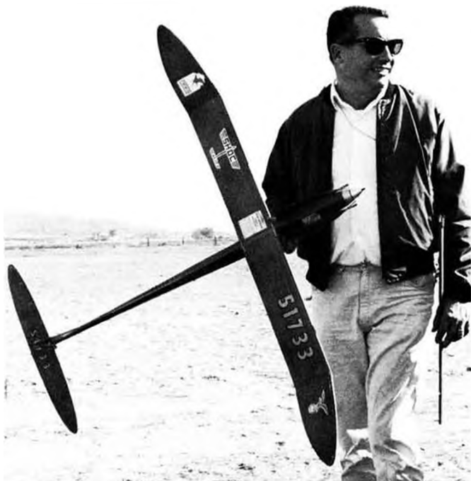
All sheet structure, plug-in wings and thread turbulators featured on this Wakefield by Jim Waters. Lake Elsinore George Bahrman photo.
