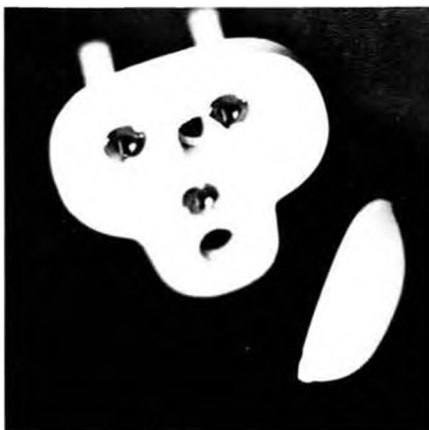
Back of firewall, showing 6-32 blind nuts and ram air duct. Looks like somebody we know.
