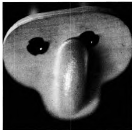
"Do you suffer from a stuffed up nose?" Ram air duct in place. Wms. Bros. makes molded one.
