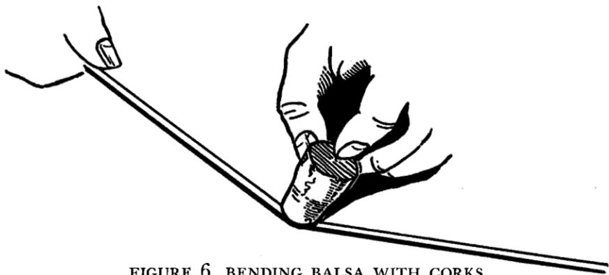
FIGURE 6. BENDING BALSA WITH CORKS
