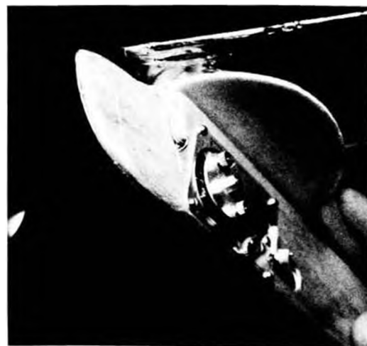
Tatone D-T timer releases "fuselage" on 8 ft. monofilament line, making wing flat spin to ground.
