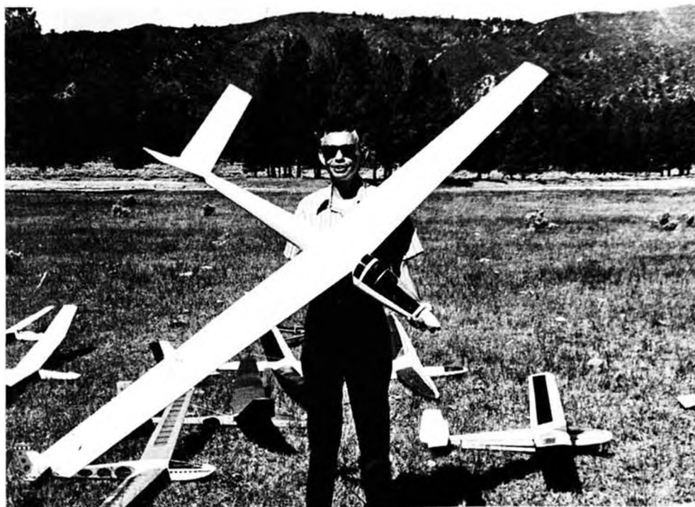
Irv Stafford, San Diego, with HP-14, built from Guenther-Wolsleger kit, which features fiberglass fuselage, machine-cut ribs, complete plans and 3-views. Kit based on John Donelson design.
