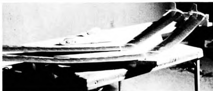
Heating and shrinking the Monokote covering while wing is on jig provides the required dihedral and washout.
