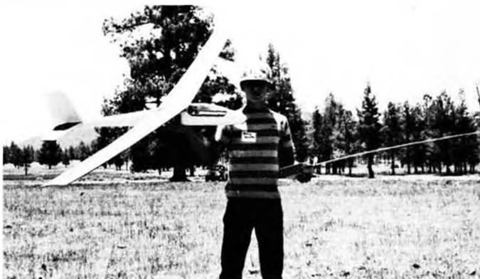
Tracy Smith and his Dart, by JP Models. Ship features rolled 1/32 plywood fuselage, which comes in kit complete and painted.
