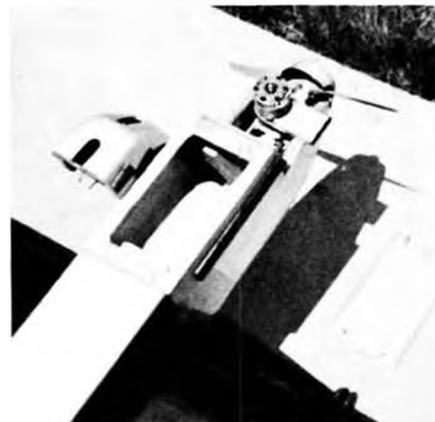
Cowl and hatch removed, it is possible to see the air ducting to the rear-rotary carburetor.
