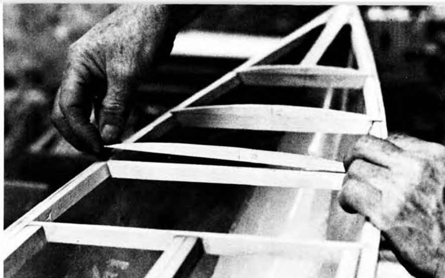
Using straight deck beams with separate curved top pieces simplifies the installation. Keeping everything level during this step is of prime importance. Make and use a rigid boat stand!
