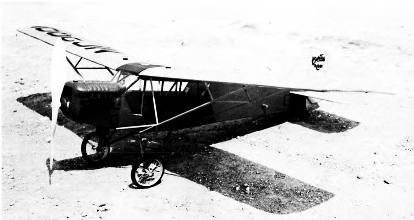
The completed Curtiss Robin, sporting FH wire wheels and Wms. Bros. prop, is an excellent flyer. Notice shim for right thrust under button.
