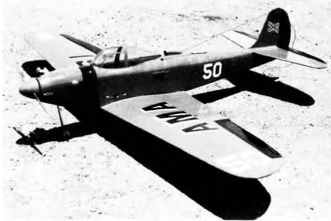
Dave Bates from Florida (!) raced at San Diego with this O.S. 15 powered P-39, scratch built from plans by Ed Nobora.
