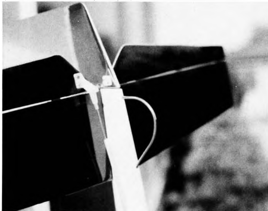
We added the 1/8 inch OD brass tube skid. Low stab position makes it extra vulnerable, especially during landings. Stab touched first when ship was at rest, actually bent it from weight.
