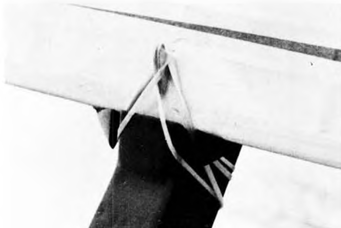
Ply "hook" on DT stab also acts as a stop, eliminating limit wire. Orbiteers are a San Diego free flight club. Bob is 1973 President.
