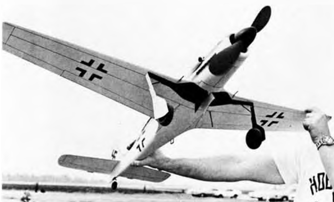
Hal Cover, designer of this month's Flapper, built and flew this beautiful FW 152. Balsa covered foam with stunning paint job.
