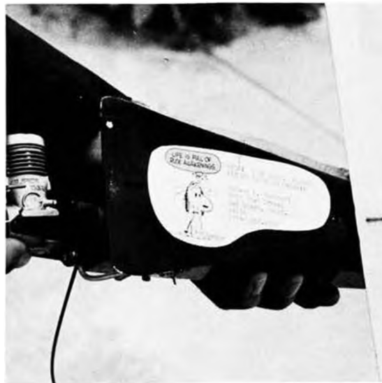
Keys are important for consistent and continued alignment. Ship is finished in black Hobbypoxy fuselage and . . . er . . . pink tissue wing and stab. Snoopy turns up just about anywhere, not so?
