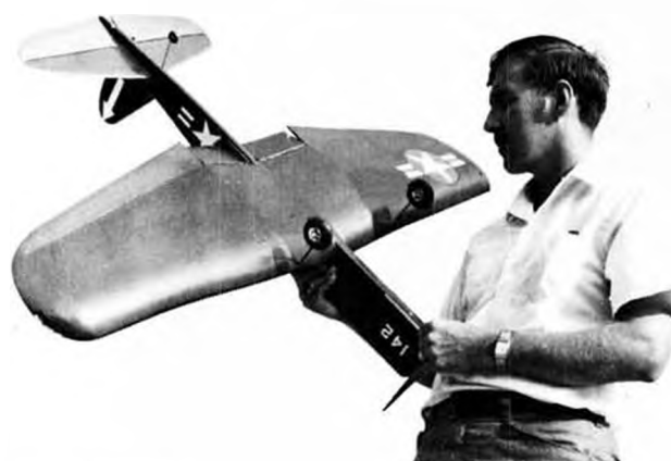
Dennis DuVall gives us a look at the underside of the profile Corsair. A Top Flite 11/6 Power Prop worked best with the McCoy 40.
