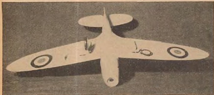
A bottom view showing the automatic landing gear extended and retracted.
