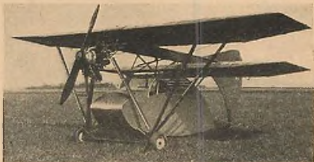
SCARABEE, novel 40 h.p. French light plane, is claimed convertible as auto for travel to airport. Parachute on back releases in flight emergency. Gross is 881 lbs., top speed 80, landing 19.
