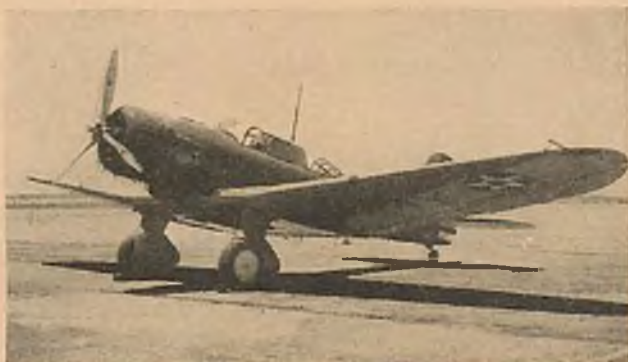
NORTHROP A-17 army attack, powered by 750 h.p. Twin Wasp Jr., has 220 m.p.h. top speed, 1,760-mile range, 20,000-ft. ceiling; five machine guns, and bomb racks. Flaps are perforated.
