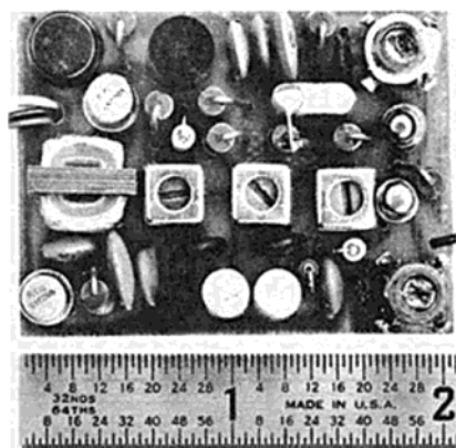
Excellent new single channel relayless superhet from Citizen-Ship.
