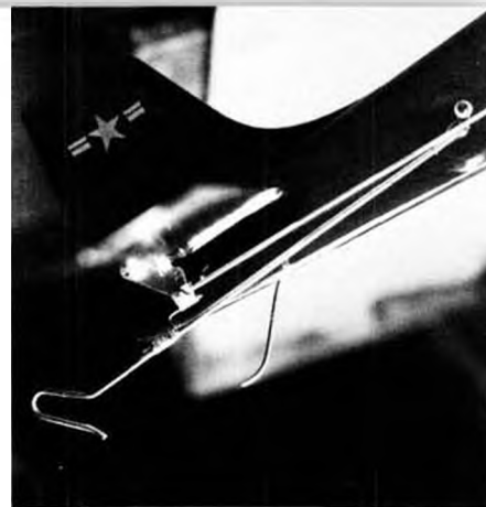
About 3/4 down elevator will release hook.
