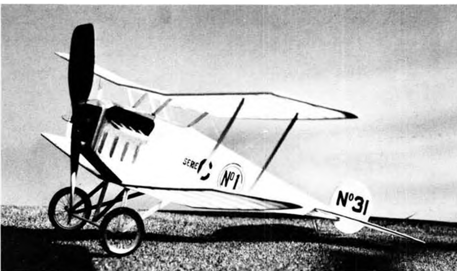
Plane's rather angular lines are sharply contrasted by the circular rudder. Walt found that said rudder had to be increased in size to eliminate Dutch roll. See text.
