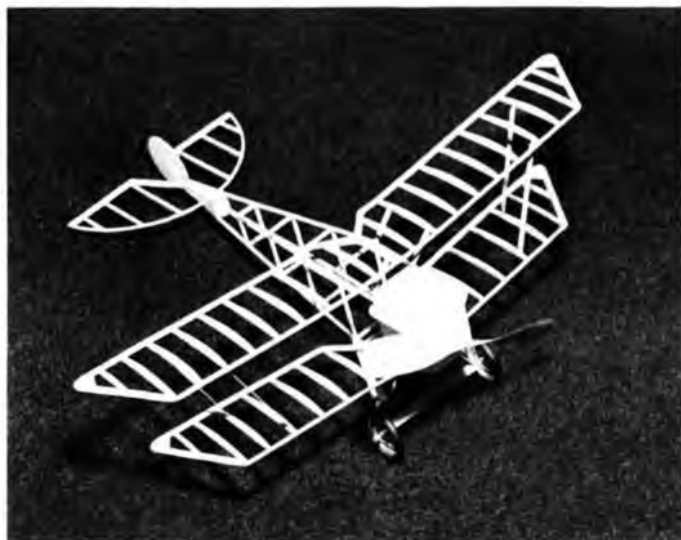
Bones of the Veloz display the easy construction resulting from its squarish lines. You may want to add a spar to top surfaces of wings.
