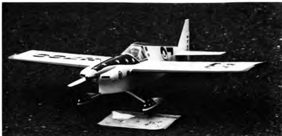
Tom Christopher's Ole Tiger Formula I. Get this! The ship was flakey in handling until after he painted on the leading edge trim! A small but effective turbulator.
