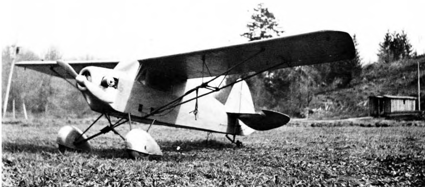
This is the plane that started control line flying in the U.S.! Oba St. Clair, designed and built the plane, flew it for the first time on July 5, 1937. The twin Forster 99 engine (1.98 cu. in.!) swung a hand carved 18 x 5 prop. The ship weighed 14 pounds, had an 8 foot span wing with 16 inch chord. It flew on 24 lb. silk lines 50 feet long, and had elevator, aileron, rudder, and throttle controls! More on this later.
