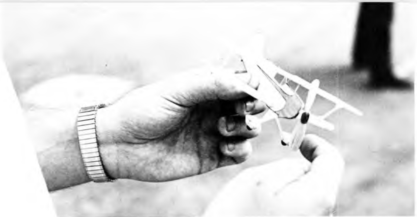
Half a Peanut is better than none! Bill Watson's little Pitts has profile fuselage, clay spinner for ballast!
