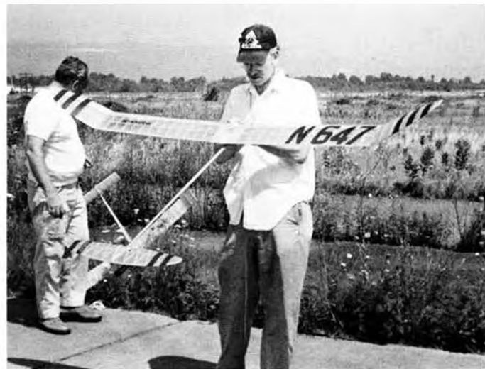
Bob Hatschek preparing his A/2 at Galeville. Circling and catapult hook is his design and product. Ship has aluminum nose.
