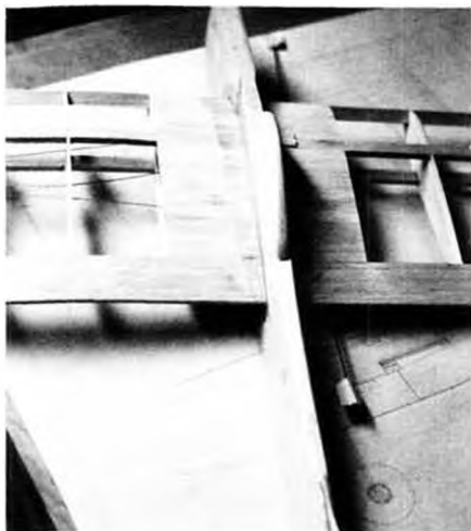
First fillet of 5-minute epoxy applied.
