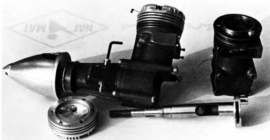
"Doc" Anderson spark ignition .49-.60, designed, built, and flown back in 1947. These are very rare collector's items.
