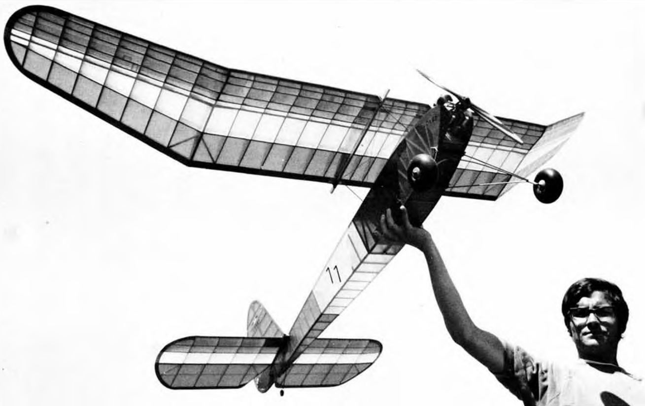
Otto Bernhardt's son Phil holds the Lanzo aloft for a through-the-covering shot. Otto added extra verticals and cross-pieces in the fuselage. Lanzo was one of the earliest to use multi-spar construction in wings and tails. The turbulator effect really pays off.
