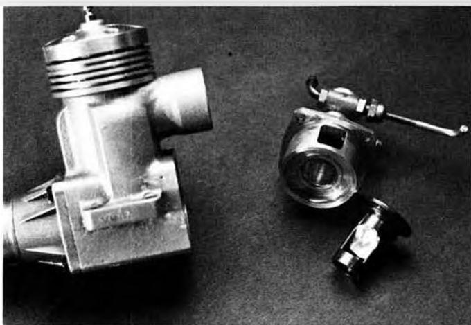
Vela T.W.A. Rossi. Backplate for housing drum rotor.
