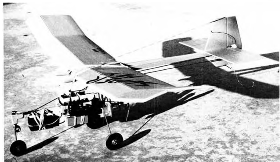
LIAHO's surfaces are all sheet balsa. Wing is Jedelsky type, but uses only two ribs at the center section. Two-channel brick radio can be used without throttle.
