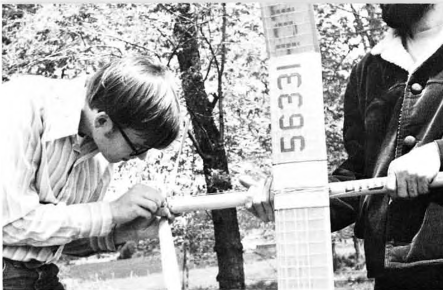
John Patchler's Wakefield uses front end assembly sold by Murry Stringer, New Zealand. Prop stop actuates auto-rudder. Ron Evans, with additional beard, holding.
