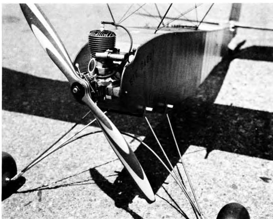
Otto used a spreader bar for more flexibility in the landing gear than would be had in the original. A beautiful carving job on that prop!
