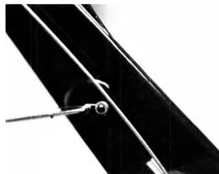
Spring forces hook down and holds it in position to catch deck lines.
